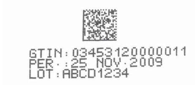
Figura 3.2.2-1 GS1 DataMatrix impreso a chorro de tinta
